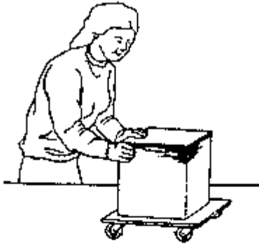
Figure 44 - Rolling platform to avoid lifting
